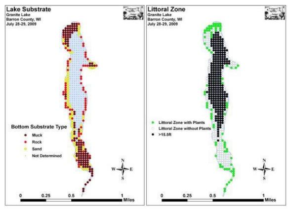
Figure 5: Granite Lake Bottom Substrate and Littoral Zone
