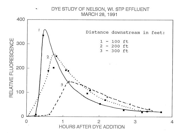
Figure 3. Results of effluent dye tracing at Nelson's Municipal Wastewater Treatment Plant in the backwater area of Pool 4, Mississippi River on March 28, 1991. 250 ml of Rhodamine WT dye added to effluent at 11:50. Samples represent surface grab samples collect 5 to 8 ft from the shoreline.
