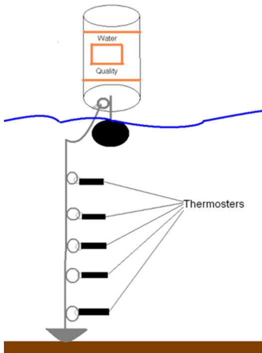
Figure 24. Diagram depicting how the thermistors were deployed at BL02 (diagram is not to scale).
