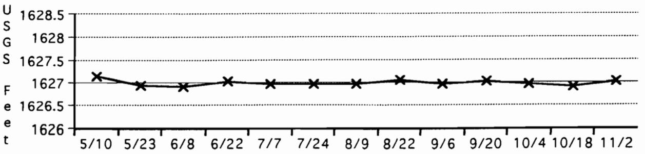
Water levels were measured from the top of the culverts. Water level of the east-west ditch was measured at the east end of the culvert beneath Thunder Lake Dam Road. Thunder Lake Dam Road ditch water levels were measured at the west culvert of the crossing, just below the location where the east-west ditch enters.
