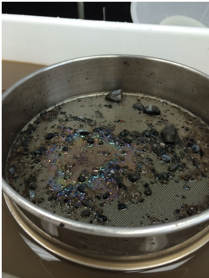
Photo 13. Sheen on sediment sieve observed during shutdown of 28 day Hyaella test at Tox Site 3.
