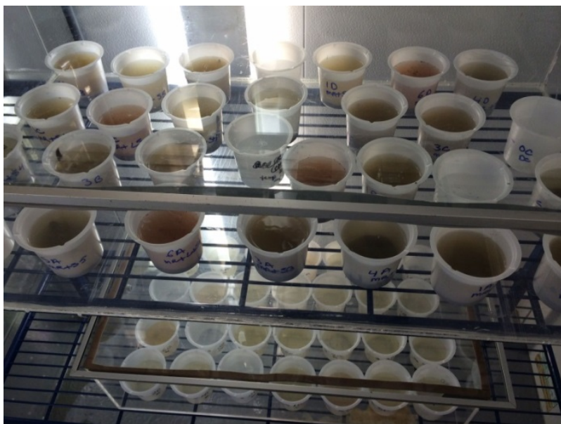
Photo 6. Acute P. promelas tests randomly set up in testing chambers.
