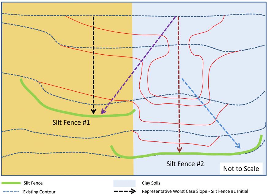
Representative Worst Case Slope - Silt Fence #1 Initial Representative Worst Case Slope - Silt Fence #1 Final Representative Worst Case Slope - Silt Fence #2 Initial Representative Worst Case Slope - Silt Fence #2 Final
