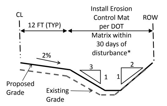
\*Disturbance may be extended to 90 days if Sediment Basin or Trap provided downstream of disturbance Assumptions:
