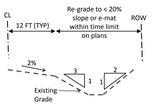
\*Disturbance may be extended to 90 days if Sediment Basin or Trap provided downstream of disturbance Assumptions:
