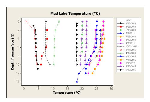
FIGURE 6. TEMPERATURE PROFILES IN MUD LAKE, 2011-2012.
