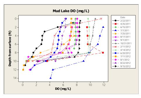
FIGURE 7. DISSOLVED OXYGEN PROFILES IN MUD LAKE, 2011-2012.
