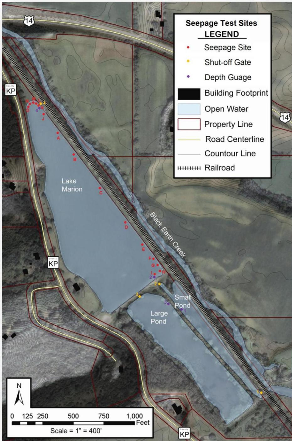
FIGURE 3.1 - LAKE SHUT-OFF AND SEEPAGE METERS SITES: MAP OF THE LOCATION OF LAKE SHUT-OFF GATES, DEPTH GAUGES AND SEEPAGE METERS. SOURCE: DANE COUNTY. BUILDING FOOTPRINTS 2009, OPEN WATER 2008, PARCELS 2009, ROAD CENTERLINES 2008, 2' CONTOURS 2009, AERIAL IMAGE 2008. CREATED BY 2010 WRM PRACTICUM.
