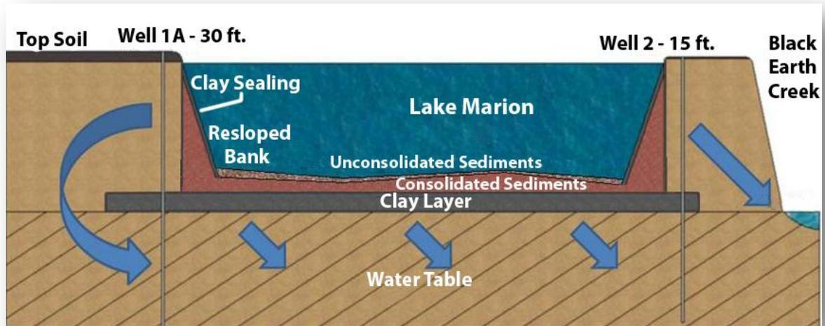
FIGURE 6.2 – SEEPAGE REDUCTION OPTIONS FOR LAKE MARION: THIS DIAGRAM ILLUSTRATES THAT THE GREATEST AMOUNT OF SEEPAGE OCCURS FROM THE EDGES (BLUE ARROWS) OF LAKE MARION. NOTICE THAT RECONFIGURING THE BANKS TO A MORE GRADUAL SLOPE AND SEALING THE PERIMETER WITH IMPERVIOUS MATERIAL (CLAY SEALING) CAN REDUCE SEEPAGE FROM THE EDGES OF THE LAKE.
