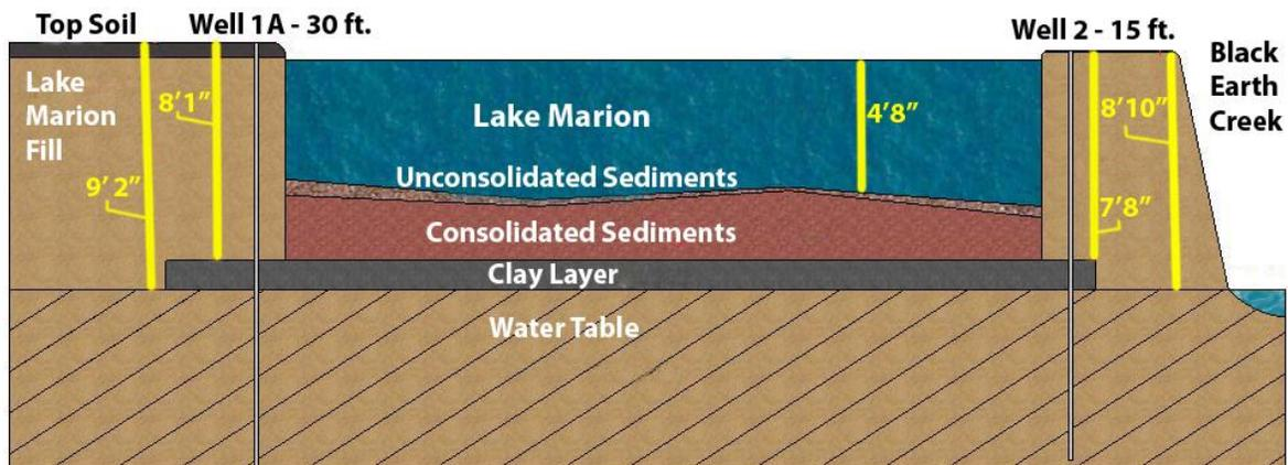
FIGURE 3.6 - HYDROGEOLOGY PROFILE: CROSS-SECTION PROFILE OF THE SOUTHERN PART OF LAKE MARION, CROSSING GROUNDWATER MONITORING WELLS 1A AND 2, BASED ON DATA FROM THE BATHYMETRY STUDY, SEDIMENT SURVEY AND HYDROGEOLOGY STUDY.
