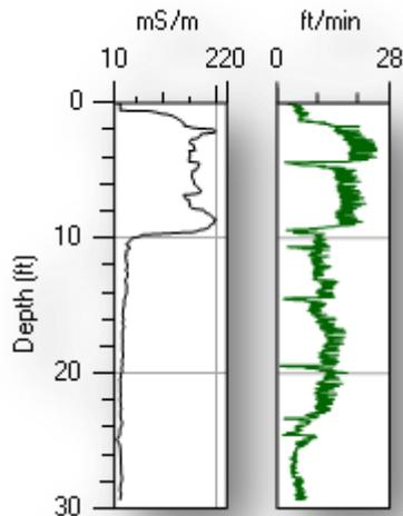
A soil conductivity profile was taken in well 1A to obtain information on the characteristics of soils around Lake Marion. The left plot (black) is electrical conductivity, in units of micro-Siemens per meter. The right plot (green) is the rate at which the probe moved through the ground, in feet per minute.
