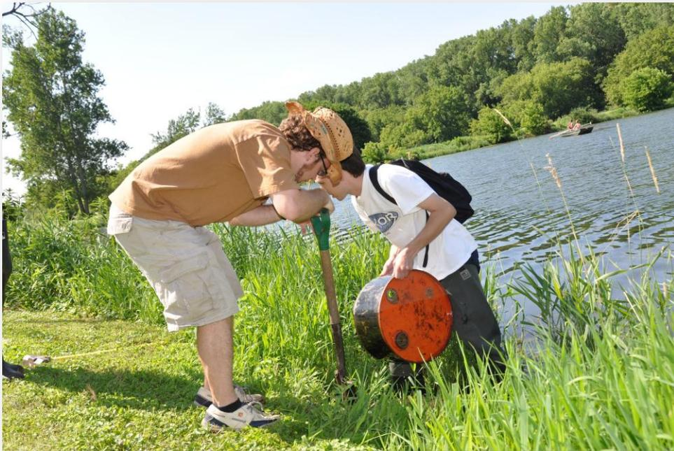
FIGURE 3.2 - SEEPAGE METER: DAVID MOSHER AND BRADLEY VOWELS INSTALLING A SEEPAGE METER ON A LAKE SIDE OF LAKE MARION.
