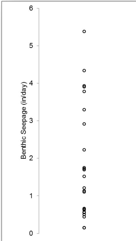
FIGURE A7.4 – BENTHIC SEEPAGE FROM SEEPAGE METERS.
