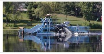
Photograph 3.3-3. Mechanical harvester.
