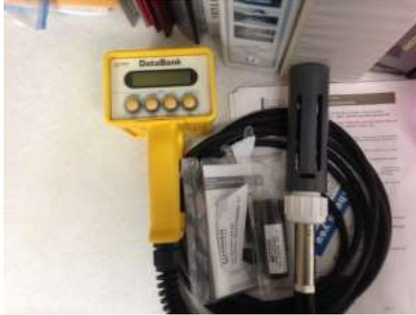
Figure 8: Turner Designs Cyclops 7 submersible sensor and DataBank® handheld datalogger used to record dye concentrations in the lake water (borrowed from the WDNR in Spooner, WI)
