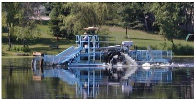
**Photograph 3.4-3. Mechanical harvester.**
