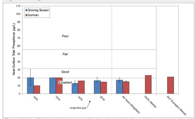
Figure 8.8.1-1. Manitowish Lake, state-wide deep, lowland drainage lakes, and regional total phosphorus concentrations. Mean values calculated with summer month surface sample data. Water Quality Index values adapted from WDNR PUB WT-913.
