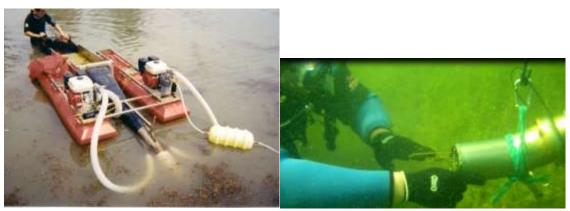
Figure 26: DASH - Diver Assisted Suction Harvest (Aquacleaner Environmental, http://www.aquacleaner.com/index.html); Many Waters, LLC)
