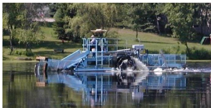
**Photo 3.4-3. Aquatic plant mechanical harvester.**
