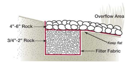
Figure 6: Rock Infiltration Set-up
