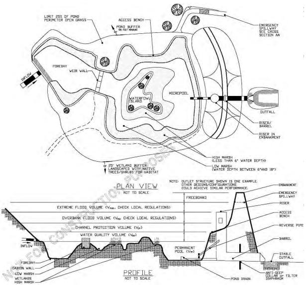
Figure 23. Design recommendations for stormwater wetlands (plan and profile).
