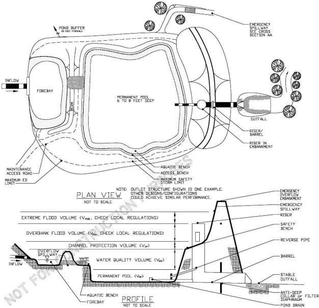
Figure 24. Design recommendations for stormwater ponds (plan and profile).
