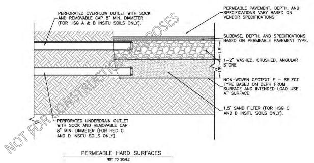
Figure 18. Design recommendations for pervious pavements.
