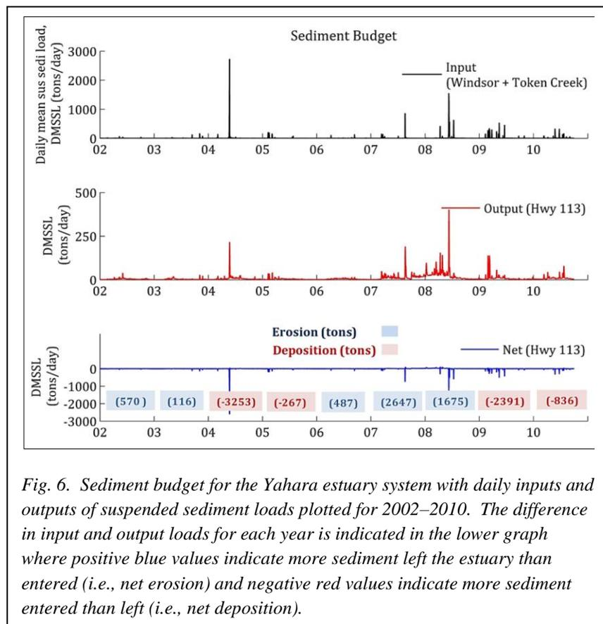
Fig. 6. Sediment budget for the Yahara estuary system with daily inputs and outputs of suspended sediment loads plotted for 2002–2010. The difference in input and output loads for each year is indicated in the lower graph where positive blue values indicate more sediment left the estuary than entered (i.e., net erosion) and negative red values indicate more sediment entered than left (i.e., net deposition).
