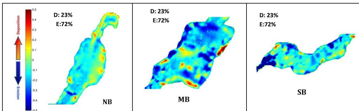
Fig. 7b. Bathymetry mapping during the second annual study period (June 2010 – July 2011); see Fig. 7a for more details. Overall, erosion predominated in all three basins during the study period.
