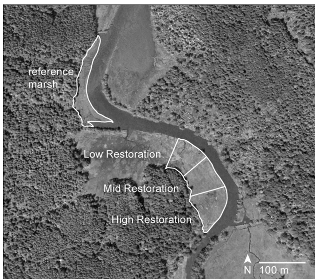
Fig. 7 At South Slough National Estuarine Research Reserve in Oregon, USA, a 10.4-ha AR experiment showed how marsh plain elevation affected tidal channel development and salt marsh restoration (treatments from Cornu et al., 2011; base image from Google Earth)
