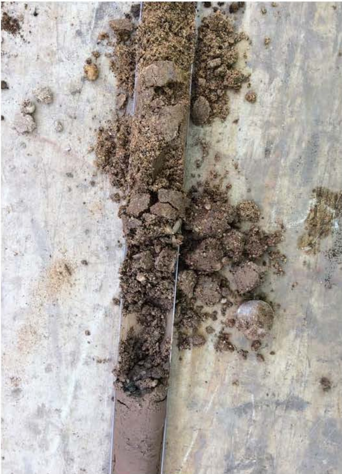
#3 - Sand/silty clay interface (typical)
