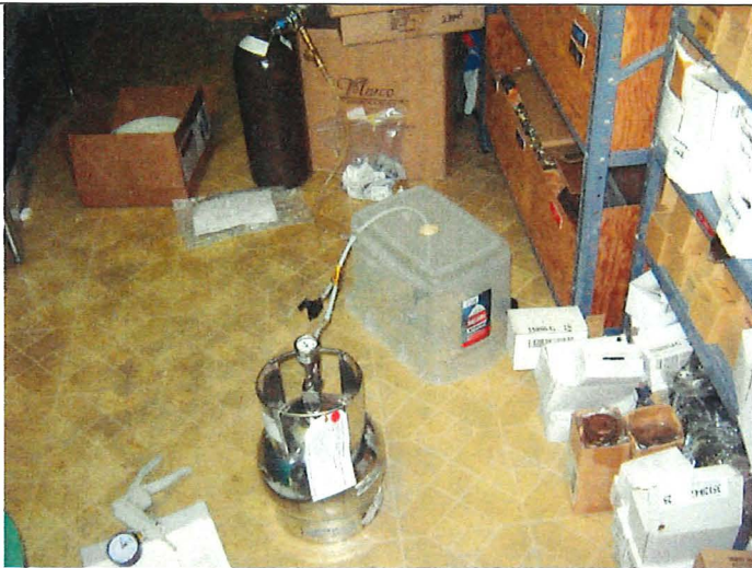
Photo 7: Sub-slab vapor sampling using 6-liter Summa canister at SSV-1.
