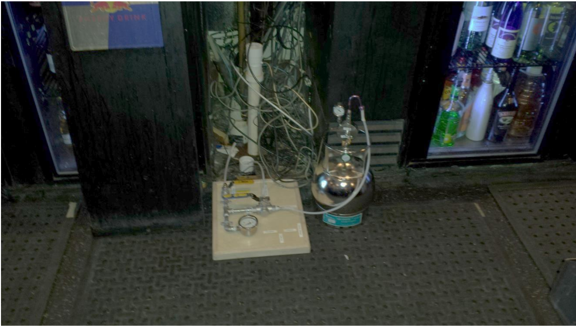
Photo 9: Cranky Pat's Sub-slab Sample SSV-6 (Bar Area)
