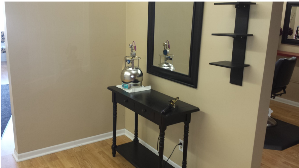
Photo 2: Village Clippers Indoor Air Sample IA-10 (Waiting Room)
