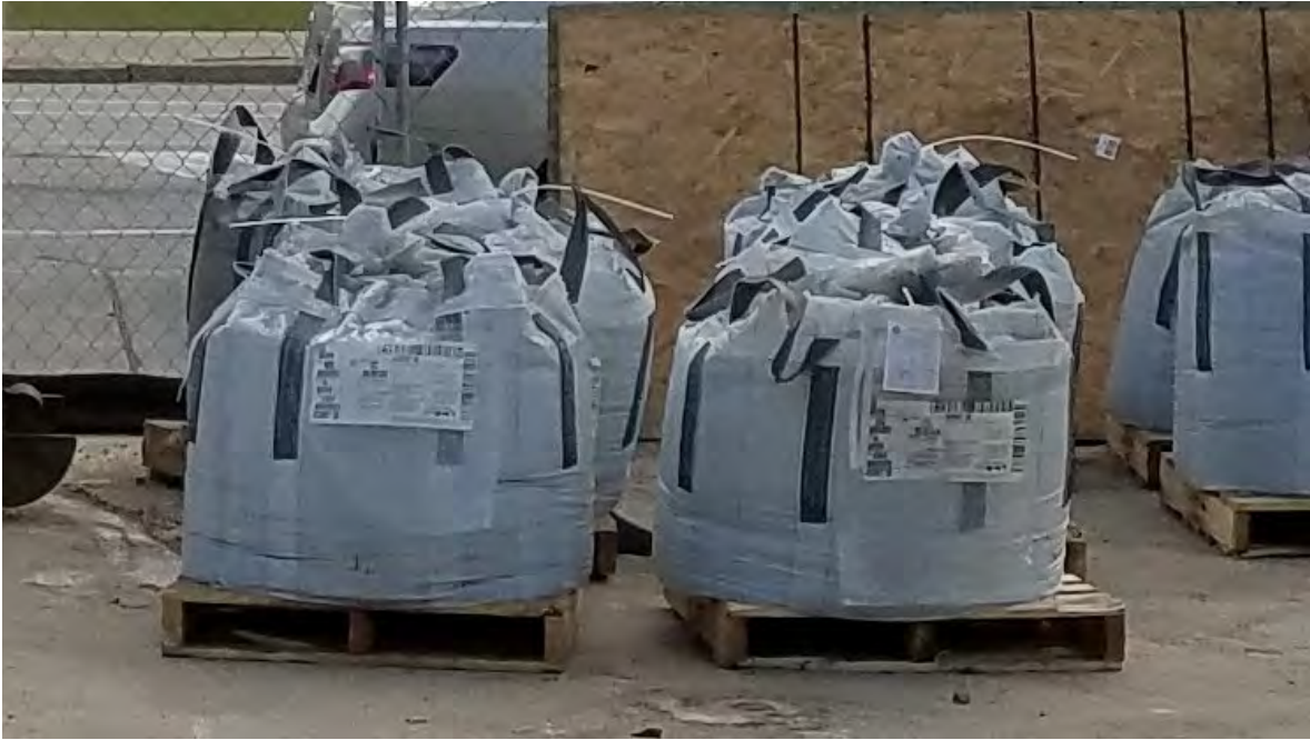
Photo 3: Typical zero valent iron woven plastic “Super Sack®”.
