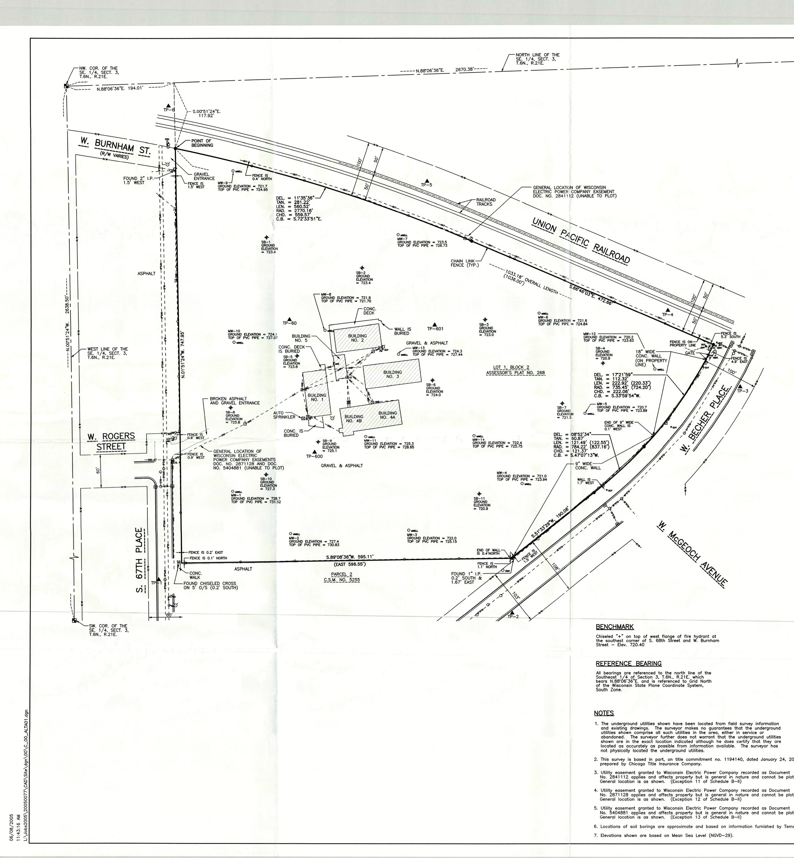
6. Locations of soil borings are approximate and based on information furnished by Temco. 7. Elevations shown are based on Mean Sea Level (NGVD-29).
