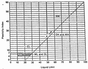
For classification of fine-grained soils and fine fraction of coarsegrained soils.
