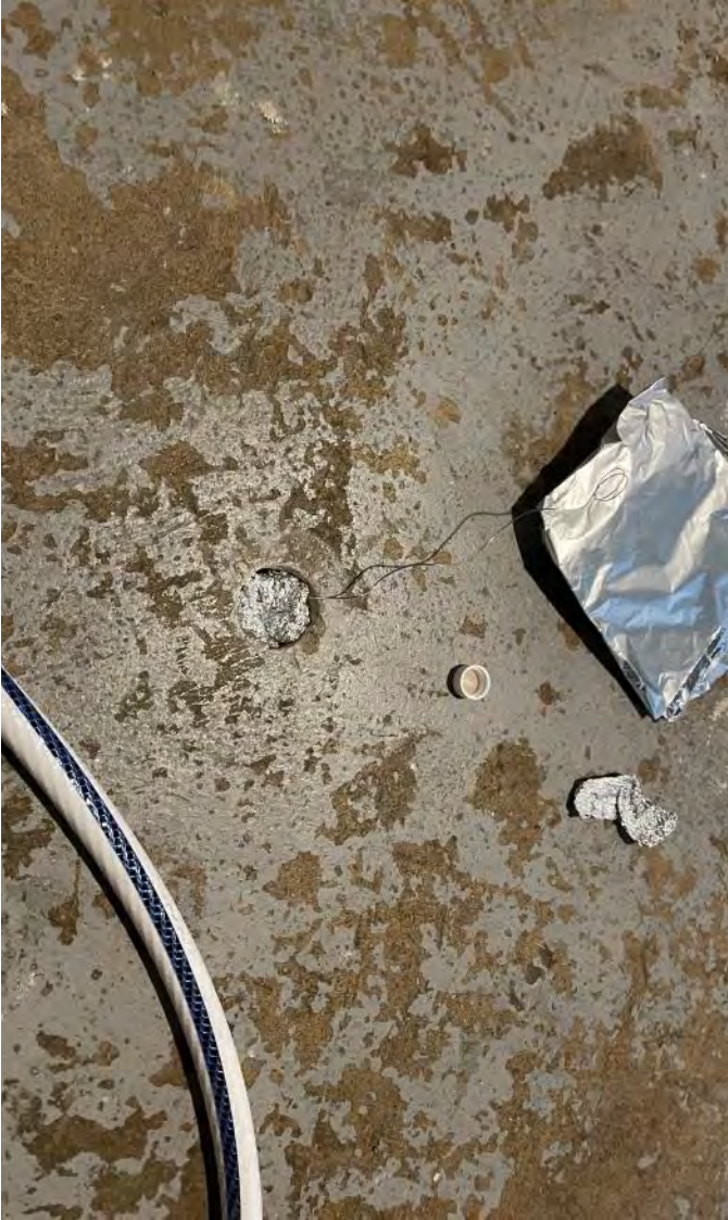
Photo 3: Aluminum foil cap installed on top of the passive Sampler near the floor crack with retrieval wire present outside of the hole. Photograph taken on June 12, 2023.
