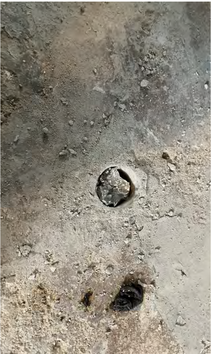
Photo 2: Aluminum foil cap installed on top of the passive sampler with retrieval wire present out side of the hole. Photograph taken on June 9, 2023.
