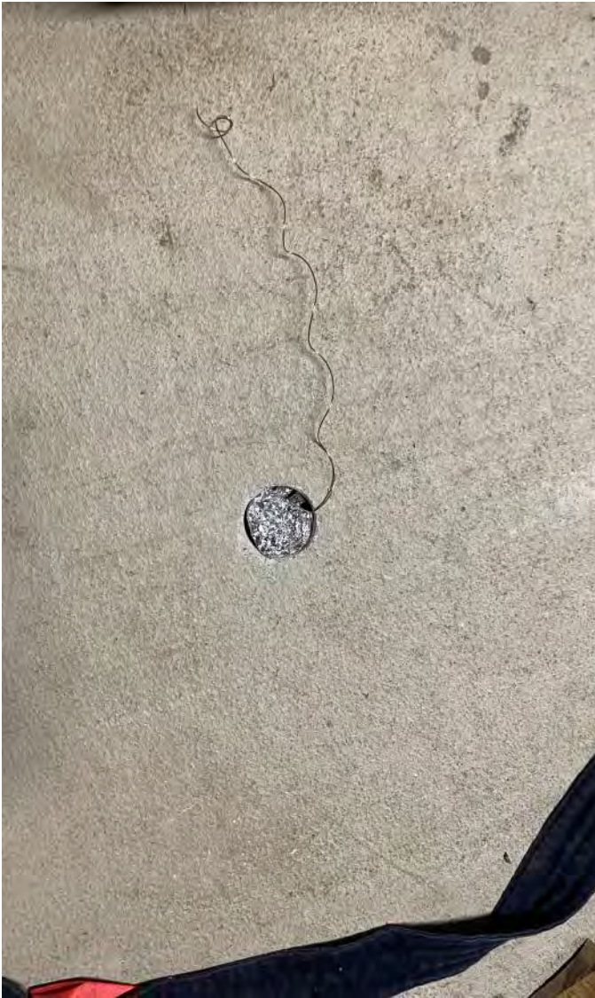
Photo 3: Aluminum foil cap installed on top of the passive sampler with retrieval wire present outside of the hole. Photograph taken on June 12, 2023.
