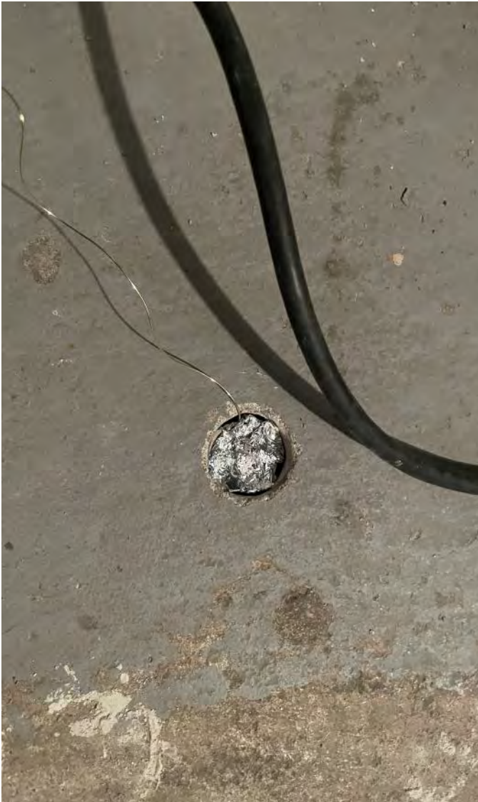
Photo 5: Aluminum foil cap installed on top of the passive Sampler on the west side of the basement with retrieval wire present outside of the hole. Photograph taken on June 12, 2023.
