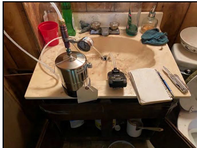
Sampling on-site sewer vapor, shop bathroom sink.
