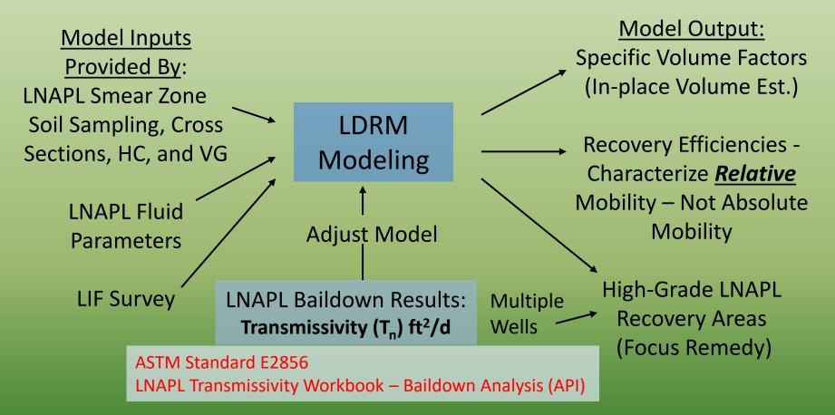
LDRM: LNAPL Distribution and Recovery Model (API) HC: aquifer hydraulic conductivity VG: vertical gradient
