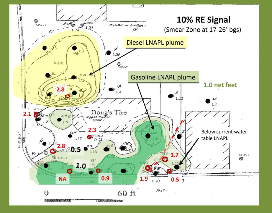
LIF results can show disconnect between true LNAPL plume thickness/distribution and that suggested by well data.
