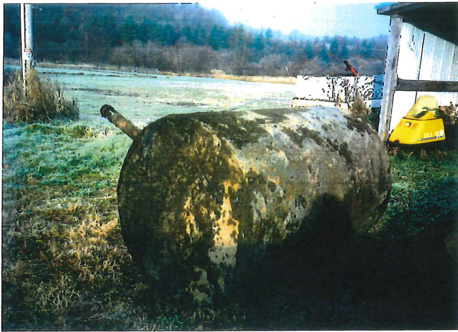
Photo C (above). View of excavated 500-gallon leaded gasoline tank. Note the tank is in fairly good condition with no obvious holes or deep pitting.
