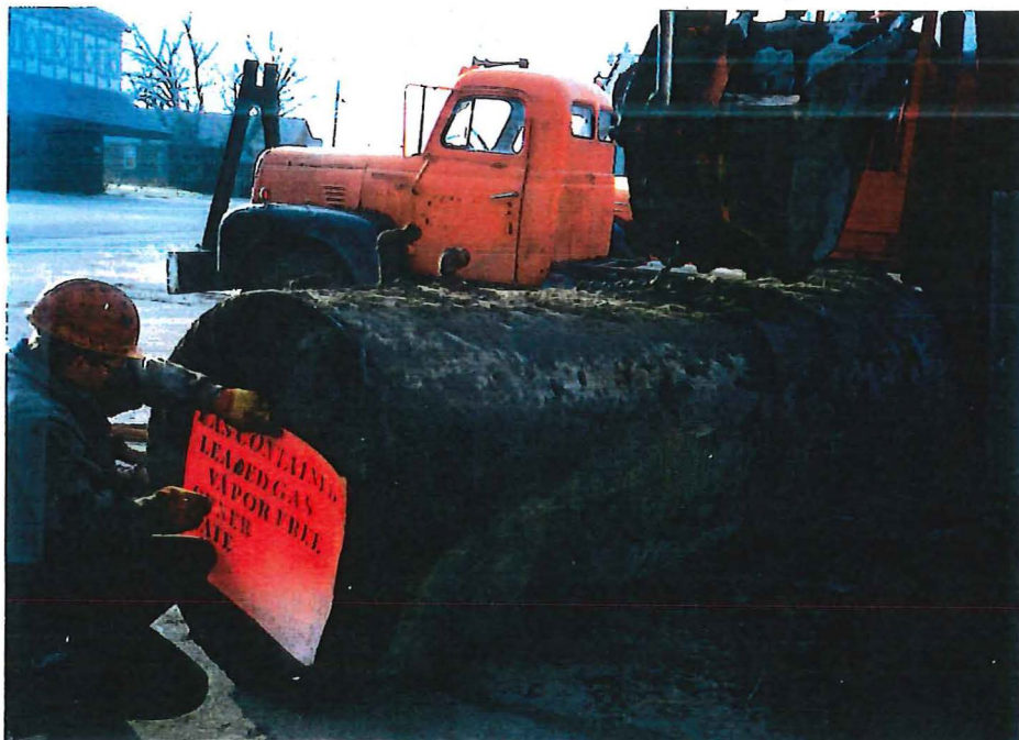
Photo D (below). View of excavated 1,000-gallon unleaded gasoline tank. Again, the tank is in fairly good condition, no obvious holes or deep pitting.
