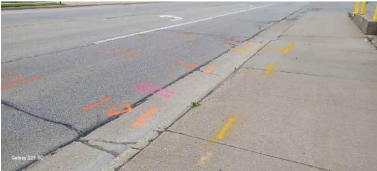
Proposed location of boring B-11 (not completed due to utilities)
