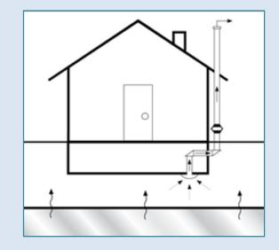
If potentially harmful chemical vapor intrusion is detected in a home or business, the most common solution is to install a sub-slab depressurization system. This system captures and redirects soil vapors from below the building foundation before they enter the indoor air. Vapors are vented outside of the building where they disperse into the air and are rendered harmless.
