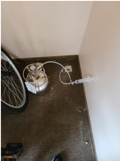
Sampling train leak test
