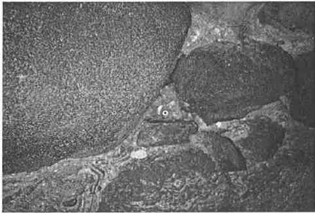
Vapor pin borehole sealed with wax
