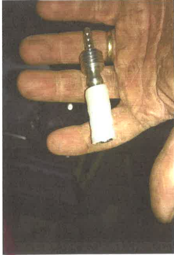
Vapor pin installed in north wall
