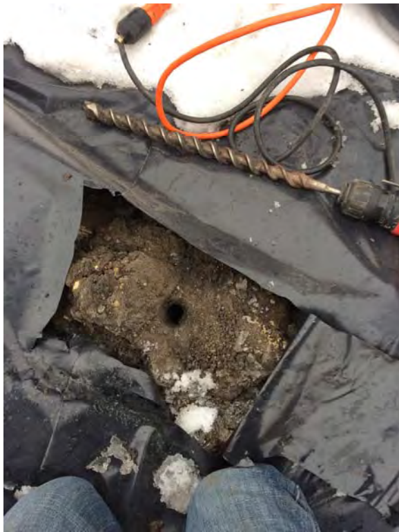
Photo 21: Sampling of treated soil in roll off boxes post-excitation.
