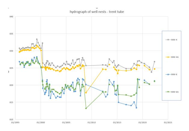
The downward gradient at the MW-4 nest, which is less than 100 feet from Honey Creek, does not support the conceptual model of an aquitard and complete hydraulic capture of contaminated groundwater by Honey Creek.
