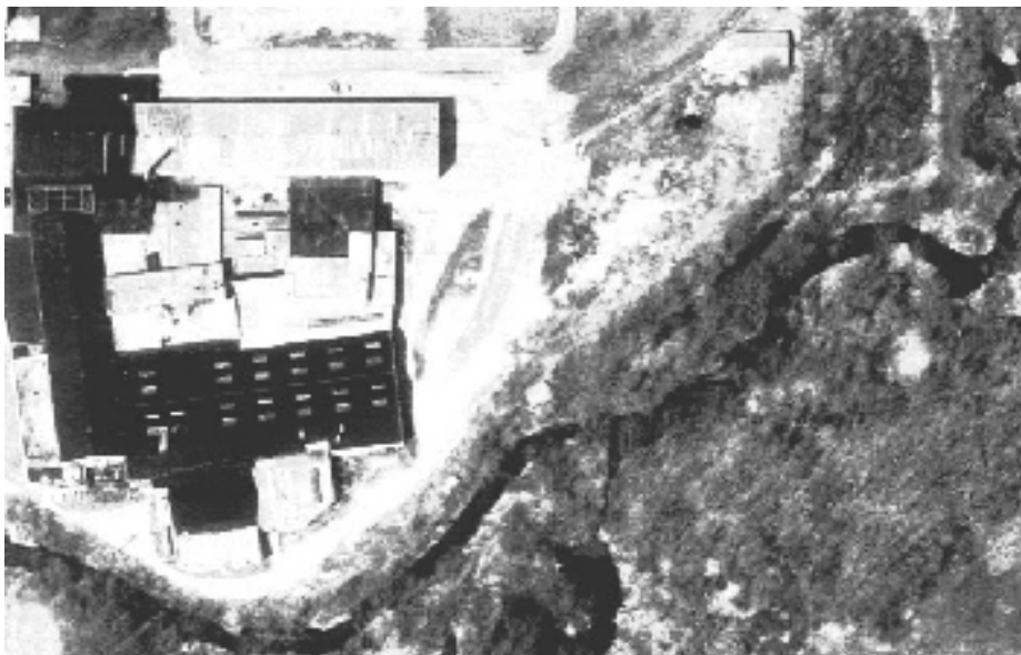
1995 Aerial Photograph showing the filled channel and lagoon covered with trees and vegetation indicating it was filled.
