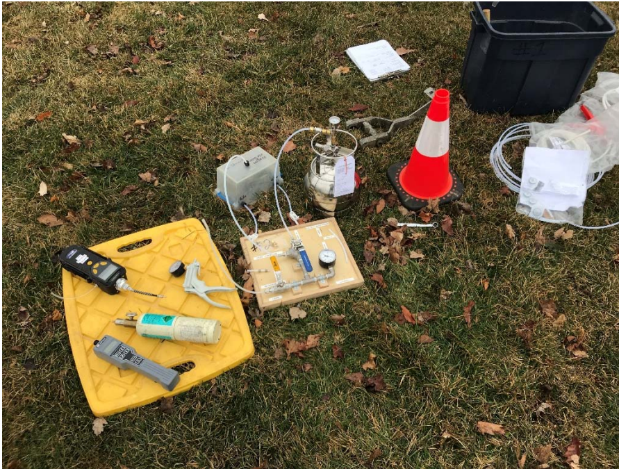
Photo 3: Sample equipment including flow manifold, helium shroud, summa canister, photoionization detector, and helium meter.
