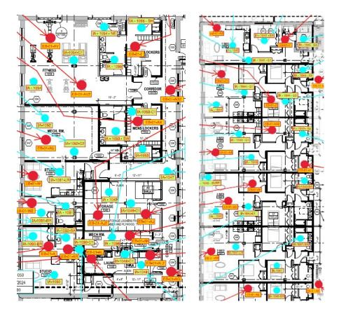
Further, as documented in Table 3 of the Report, GC samples were collected in bathrooms and showers and at columns, sumps, and elevators, all of which present potential preferential pathways for vapor intrusion. GC samples taken from locations presenting preferential pathways have the following sample ID suffixes:
