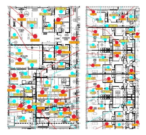
Further, as documented in Table 3 of the Report, GC samples were collected in bathrooms and showers and at columns, sumps, and elevators, all of which present potential preferential pathways for vapor intrusion. GC samples taken from locations presenting preferential pathways have the following sample ID suffixes:
