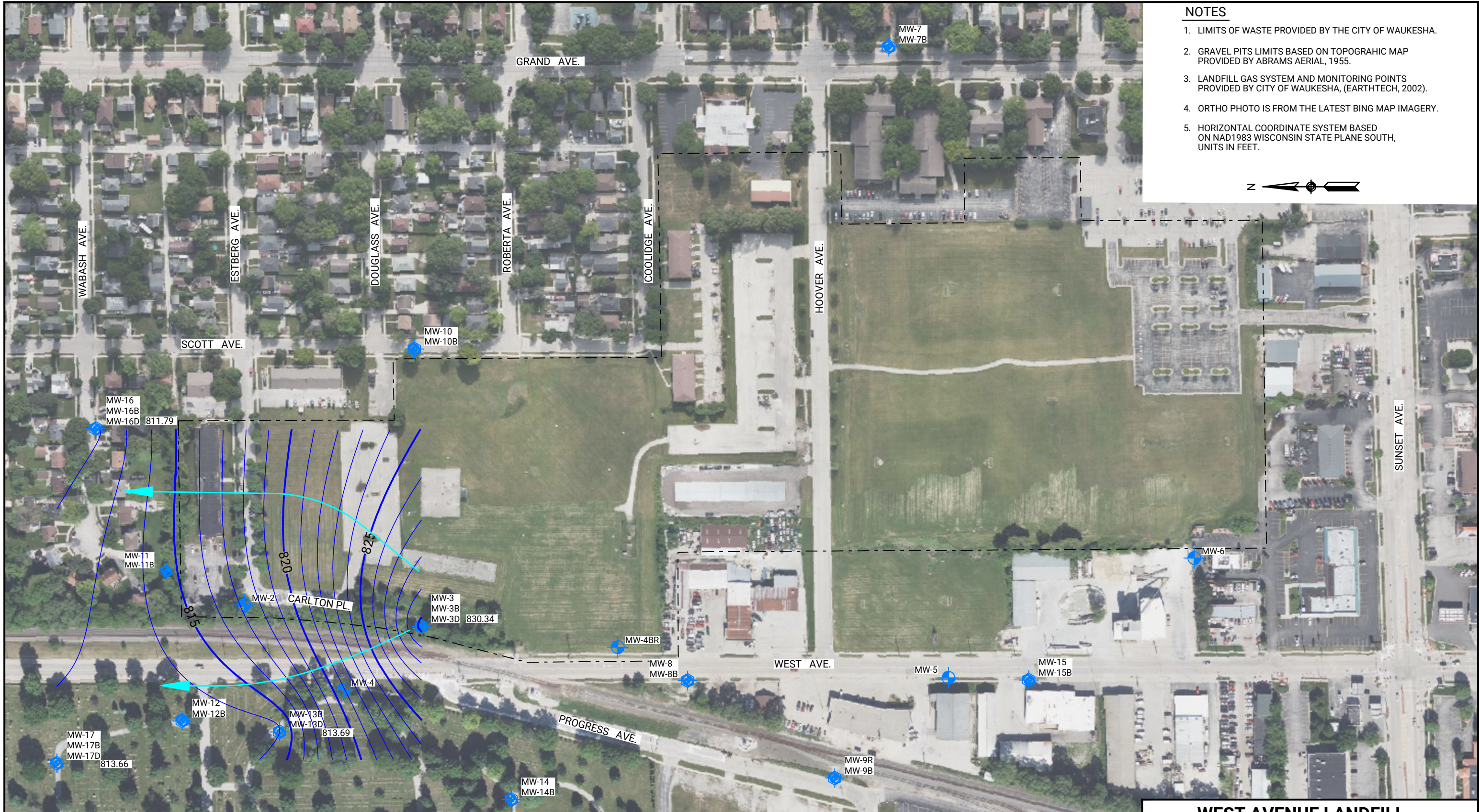
FIGURE 6 DEEP BEDROCK GROUNDWATER PIEZOMETRIC SURFACE MAP - SEPTEMBER 2022 CITY OF WAUKESHA
