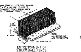
SILT FENCE ALTERNATE "B"
