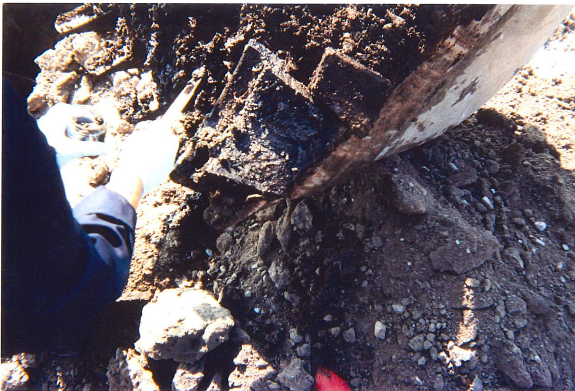
Photo 5: View of material in backhoe bucket, and collection of sample for lab analysis.
