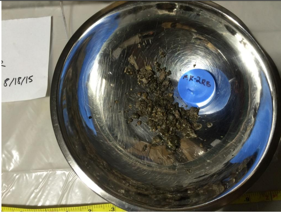
Photo 9: View of sediment from core MR2-IC-502R. The sediment shown is coarse gravel from the 0.0" – 3.6" interval which was not included in the sample.
