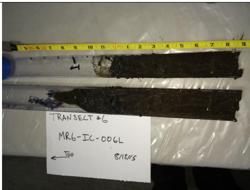
Photo 22: View of sediment core MR6-IC-006L.
