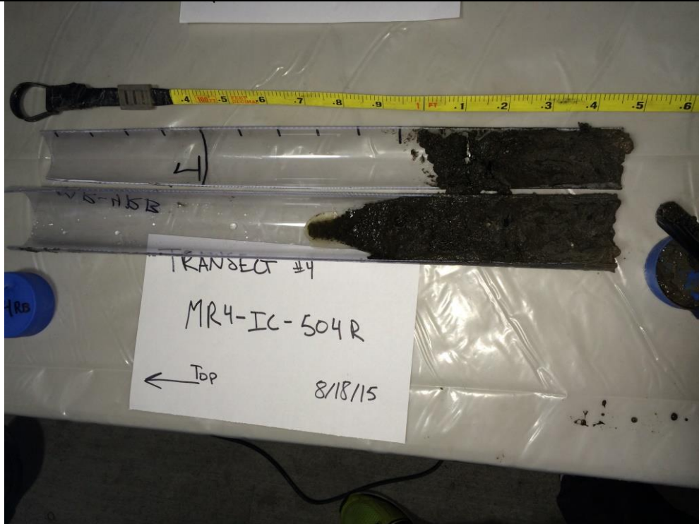
Photo 16: View of sediment core MR4-IC-504R.
