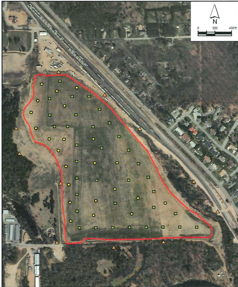
figure 3.1 CONCEPTUAL PASSIVE VENTING SYSTEM HOLTZ KRAUSE LANDFILL Wausau, Wisconsin
