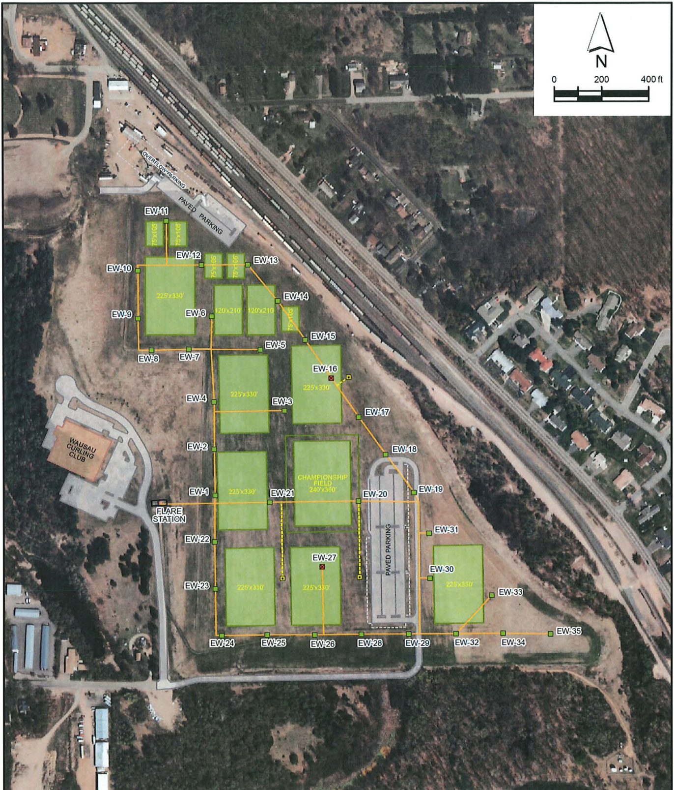
figure 5.1 CONCEPTUAL ACTIVE GAS EXTRACTION SYSTEM LAYOUT HOLTZ KRAUSE LANDFILL Wausau, Wisconsin
