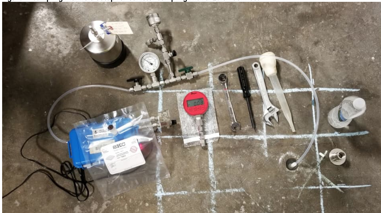
Figure 2. Sampling Manifold Setup for Canister Sampling with a Quick-Connect
