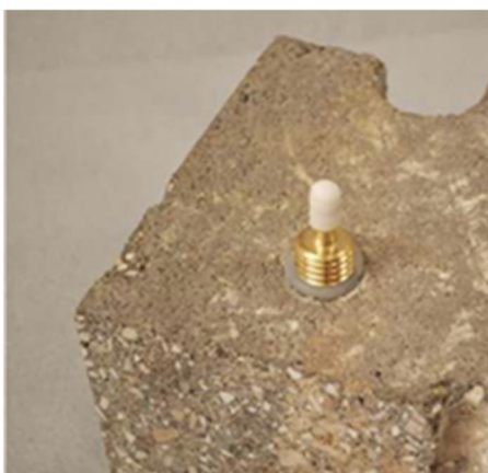
Figure 2. Temporary Stick-Up Vapor Pin
