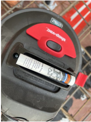
Photograph 7: Smoke Used for Vapor Barrier Testing
