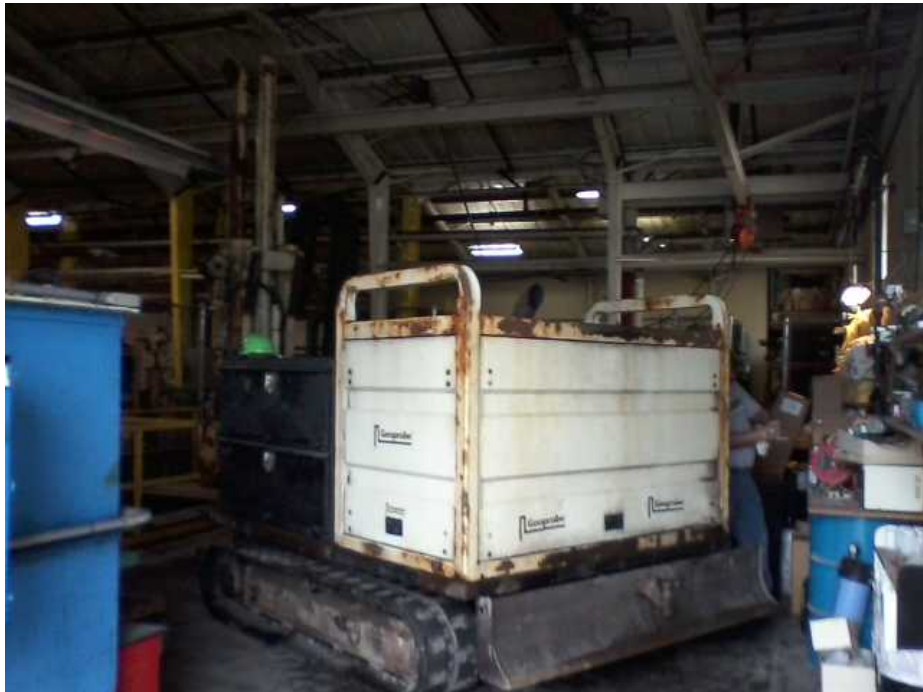
Geoprobe rig positioned on groundfloor above basement
