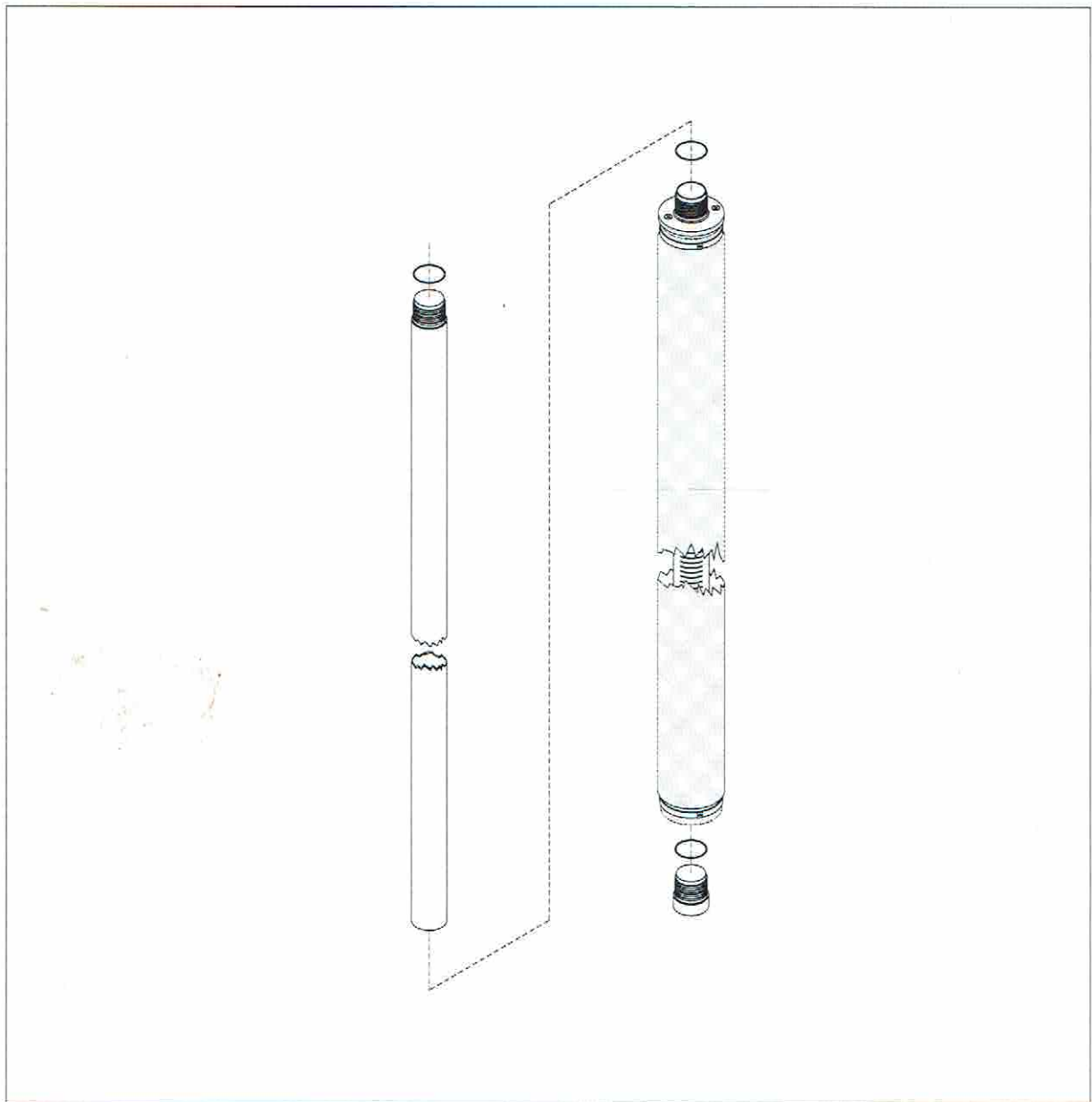
GEOPROBE® 1.0-in. x 2.5-in. O.D. PREPACKED SCREEN AND PVC RISER
