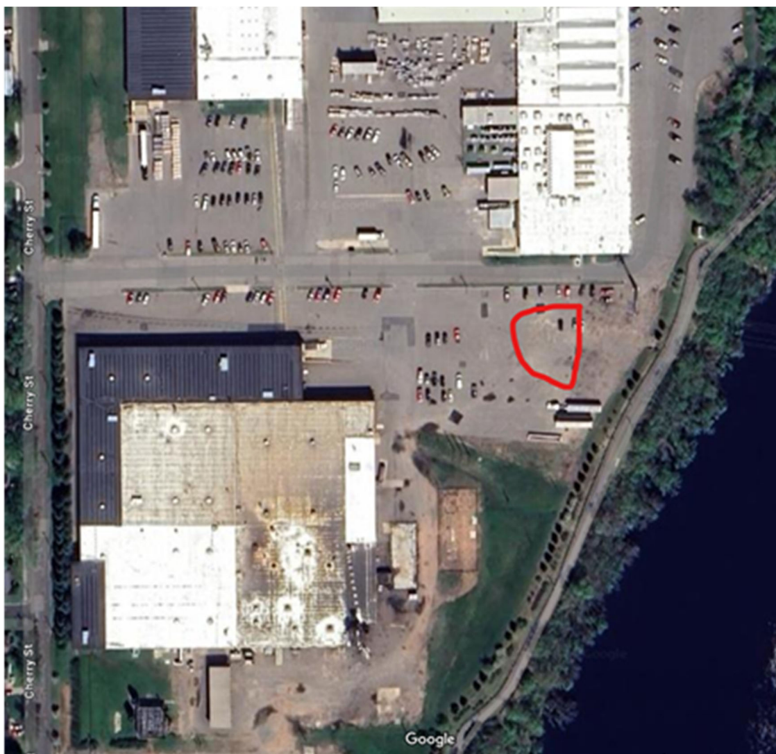
Figure: Map provided by the PRP to show areas of landfill cap with ponding, cracks, and settlement.
